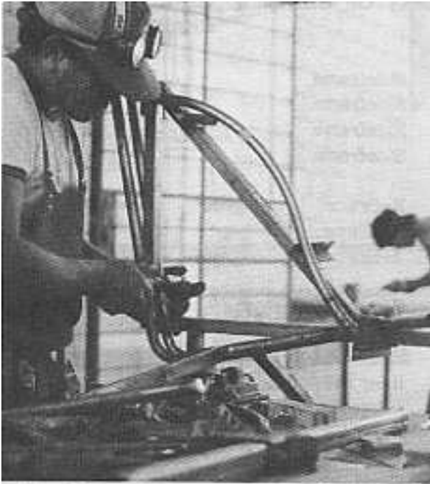
Juan Becerra of Peru Using a Sideframe Jig
